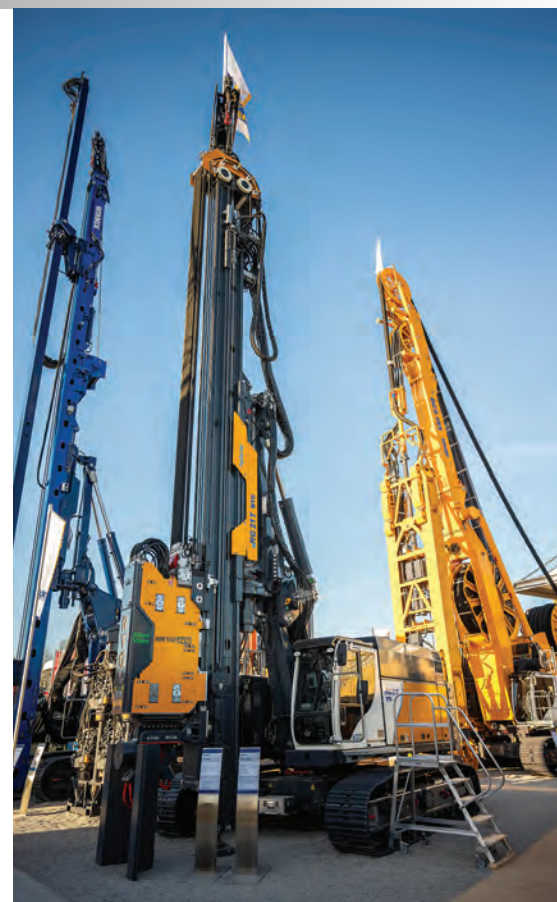
OPPOSITE: The eRG 21 T hybrid pile driver combines the power of a diesel engine and an electric motor.
