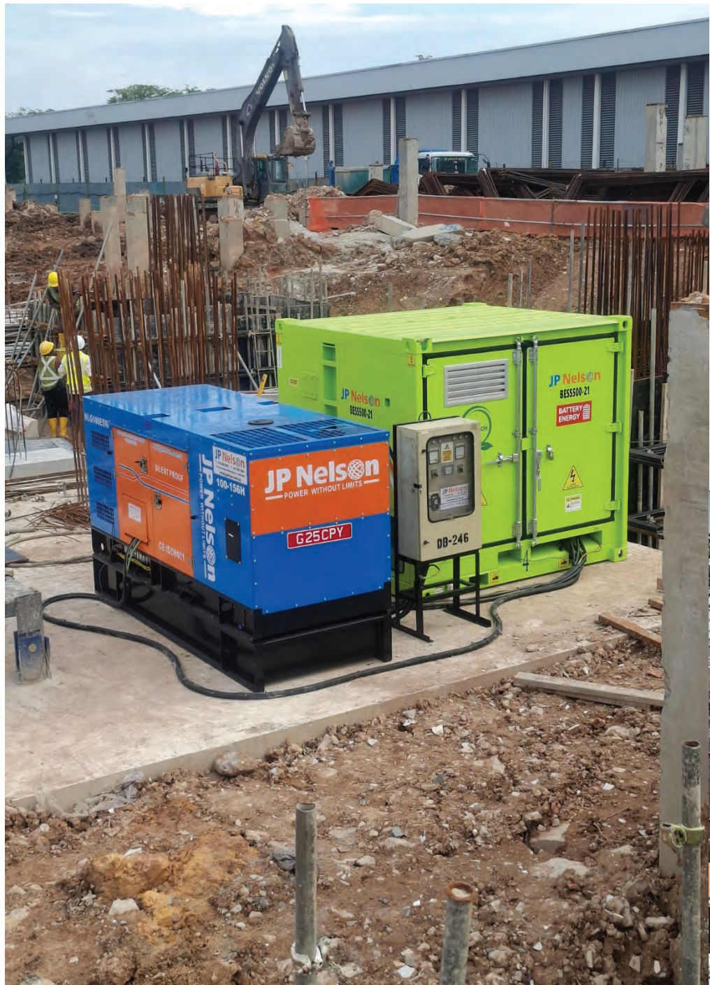
ABOVE AND LEFT: JP Nelson has deployed several units of its battery energy storage system (BESS) on construction sites in Singapore. This system is environment-friendly, reducing reliance on fossil fuels and greenhouse gas emissions. It also enhances the reliability of renewable energy sources.
