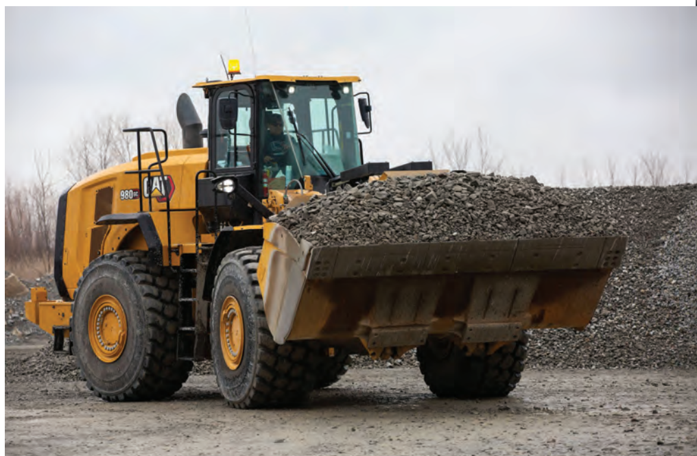
TOP AND ABOVE: With a bucket capacity range of 4.3-5.8 cu m, easy-to-load Cat Performance Series buckets use a system-based approach to balance bucket shape with the machine's lift and tilt capacity, weight and linkage.
