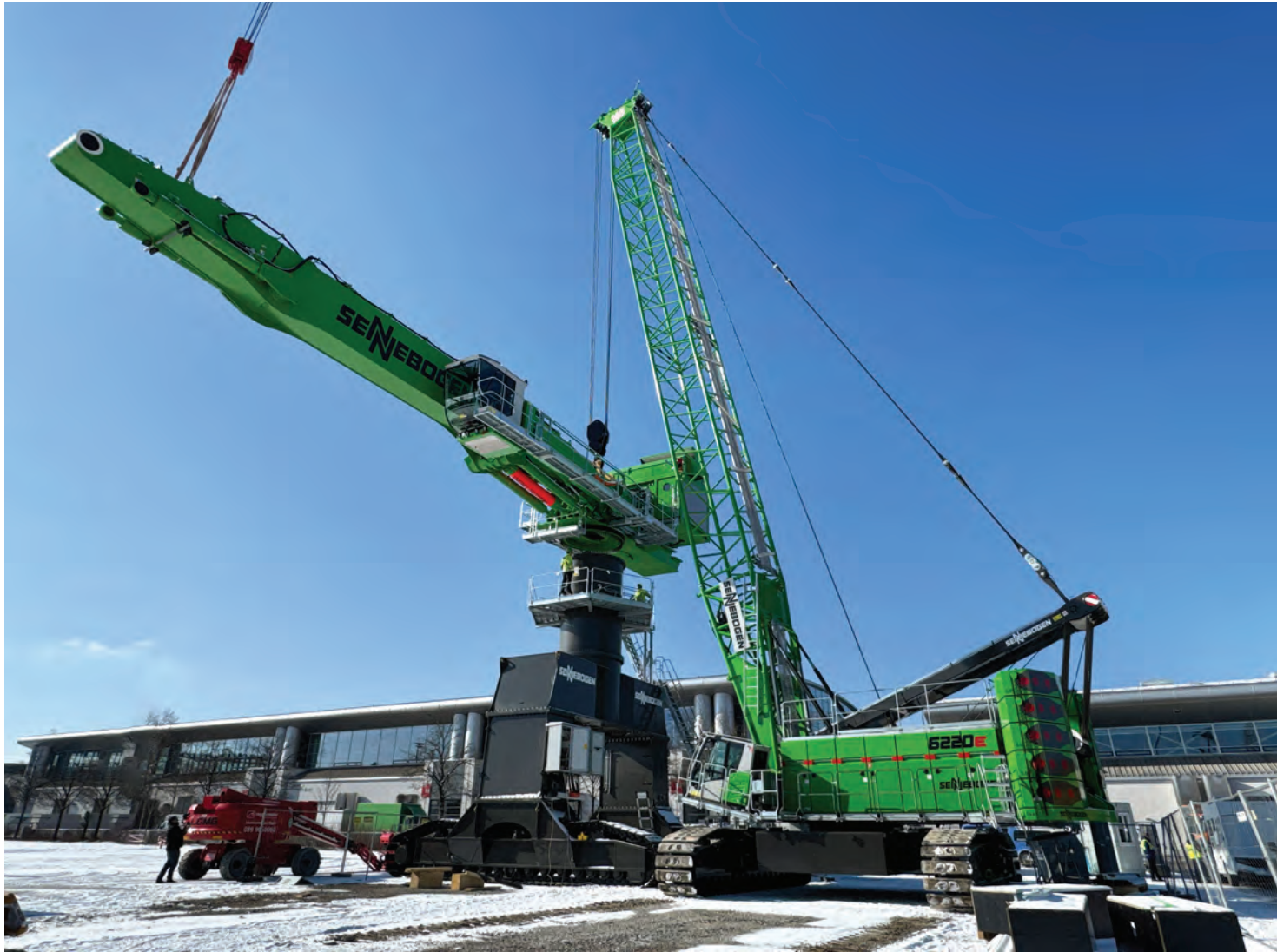
Thanks to its robust design and considerable load capacity, the 6220 E can operate under tough conditions. This duty cycle crane features a maximum boom length of 74.7 m in lifting mode.
